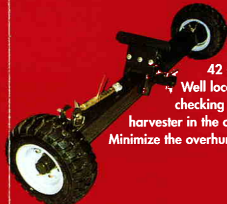
The hydraulic locker "fork" is well located under the header. You can hook it perfectly on its trailer without angle problem, without physical effort and without any risk taken by the operator who can do it easy from the seat of the Forage Harvester.
